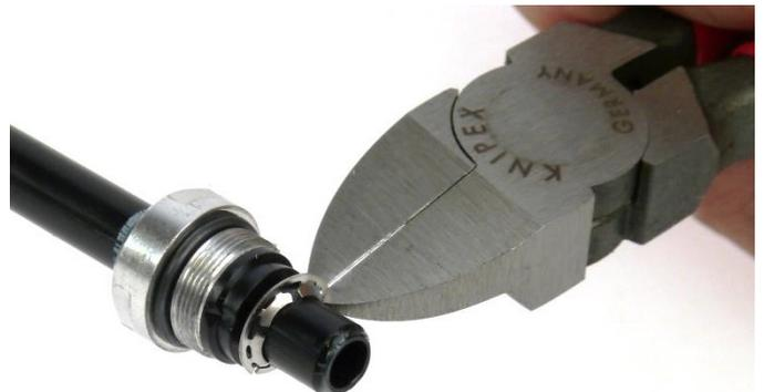
Fig. 20: Cutting the grip disc at the opposite position
