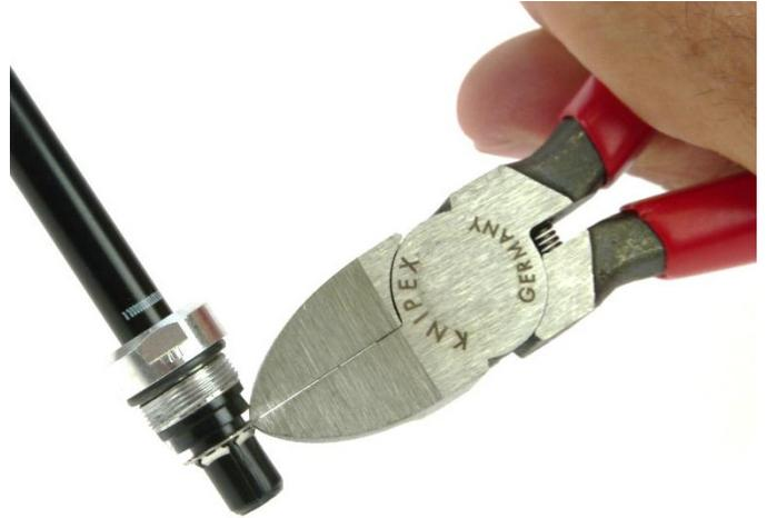
Fig. 19: Cutting the grip disc
