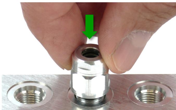
Fig. 9: Positioning the quick connector at right angles
