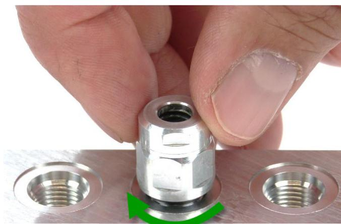
Fig. 10: Screwing in the quick connector manually
