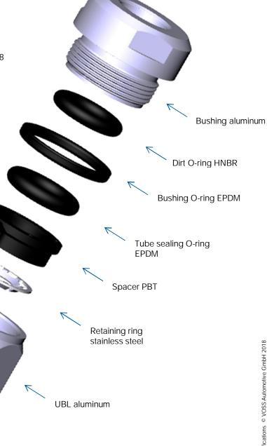
Thread-sealing O-ring EPDM
