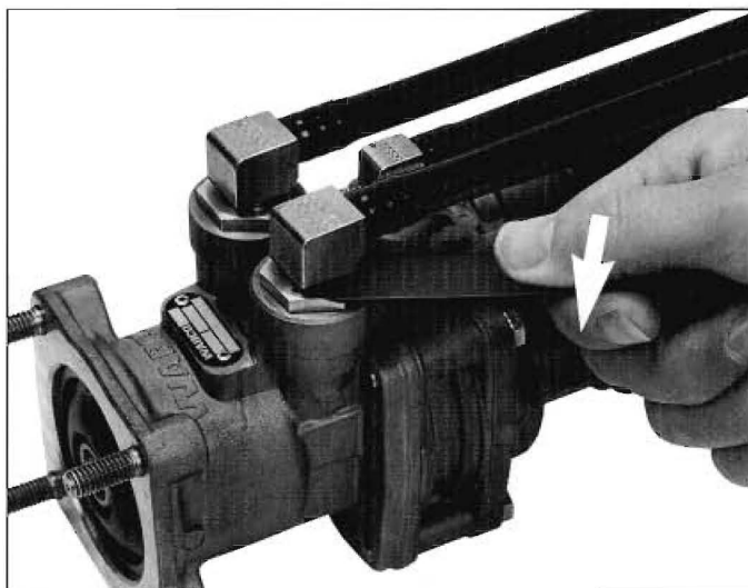
Final check with testing tool
